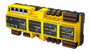
The modular concept of modulo 6 offers flexible configuration and tailor-made performance. The modules have pluggable spring-type terminals and can be lined up in front of each other. A total of up to 24 modules (I/O and COM) are possible.
