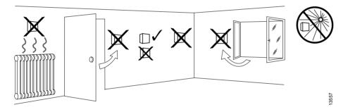
Also, air flowing from the ducts and pipes of the electrical installation can cause measuring errors. Empty pipes and installation pipes should therefore be well sealed.
